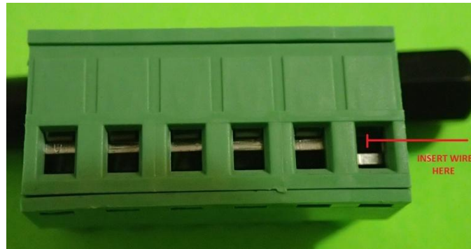
Figure 19 - Lowered metal plate for wire insertion
