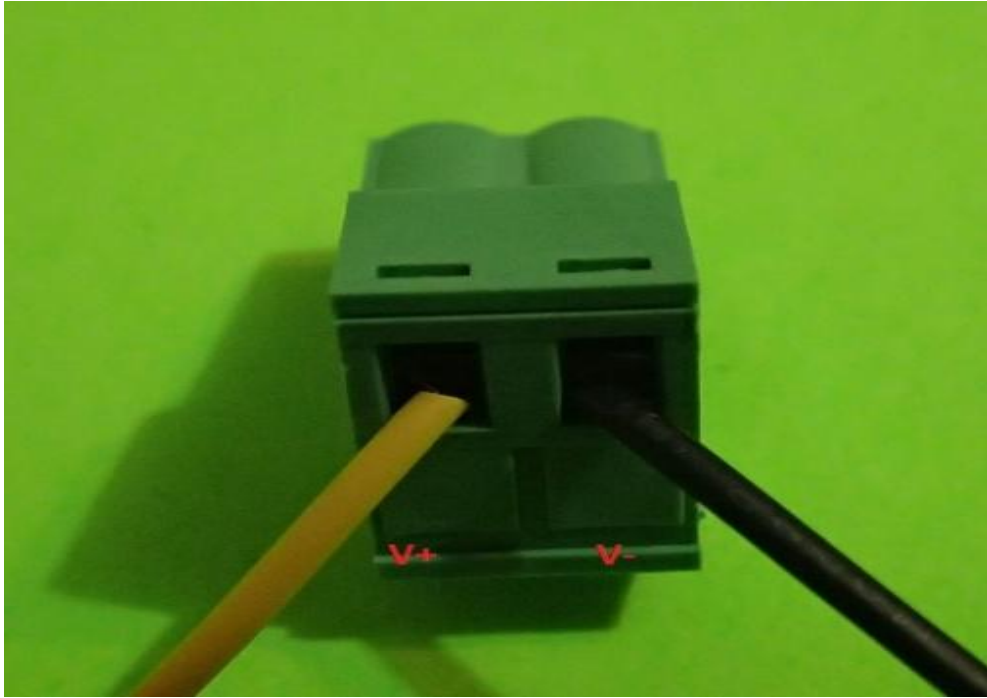
Figure 25 - Connector with wires and polarity labels
