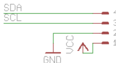
Figure 57 - I2C Expansion schematic
