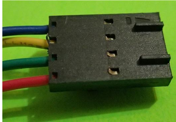
Figure 17 - Connector housing with all crimp pins inserted in the correct order
