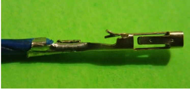
Figure 15 - Result of crimped wire with needle-nose pliers
