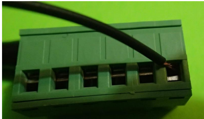
Figure 20 - Wire inserted in the appropriate gap of connector before tightening of the screw
