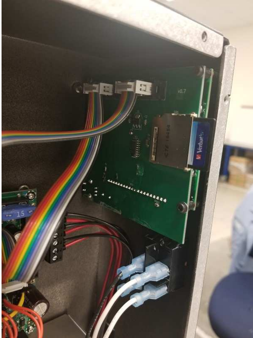
Photo #4 – Internal View of Display PCB
