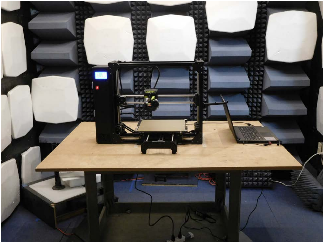
Test setup for Radiated Emissions - usb
