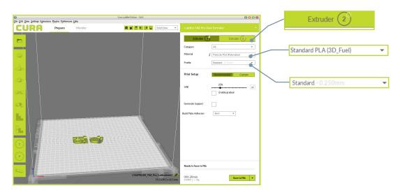
**4.7** Click on the TAZ\_Pro\_Calibration02.stl model on the virtual print bed, then click on the 2 on the left side of the print area. This designates TAZ\_Pro\_Calibration02.stl as the piece to be printed with the Extruder 2. The model with change color based on the filiment selected for Extruder 2 to reflect the change.
