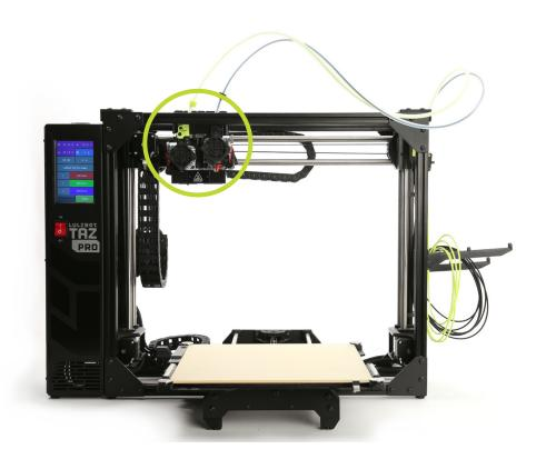
**b.b** Once each hot end reaches its wiping temperature, the Tool Head will move to the wiper pad, cleaning the nozzles of residual filament. After each nozzle has been cleaned, your LulzBot TAZ Pro will heat to probing temperature and conduct an automated self-leveling sequence by touching each of the four bed corners. When the leveling process is complete, the printing process will commence.
