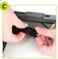
Once all connections are in place, locate the bed power harness retention clip in your tool bag. Press the two prongs of the clip into the two holes on the heater connection.
