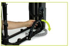
If the Y-axis cable chain does not rotate back and downward easily, loosen the screw at the base of the cable chain to allow for easier adjustment.
