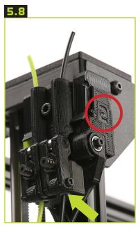
Note that the filament sensors 1 and 2 correspond to Extruder 1 and Extruder 2 and must go to the correct extruder in order for your TAZ Pro to function properly.
