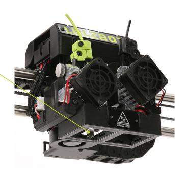
**5.4** Once the hot end reaches the appropriate filament removal temperature, press the **Continuous** button in the **Unload** column to start retracting filament. Once the filament stops moving, pull it out of the idler. Press the **Continuous** button again to stop the extruder. Select the **2 button** and repeat this process for **Extruder 2**.
