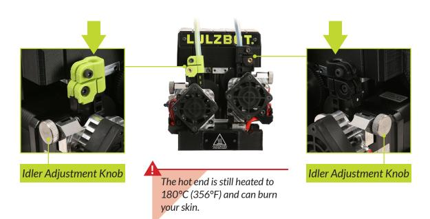
During printing, each extruder idler holds filament against the extruder hobb wich pushes filament down into each hot end. **Correct tension is important** for keeping filament flowing properly during the printing process. **Loosen** the filament tension knob **clockwise** all the way out and then tighten it by rotating **counterclockwise**.
