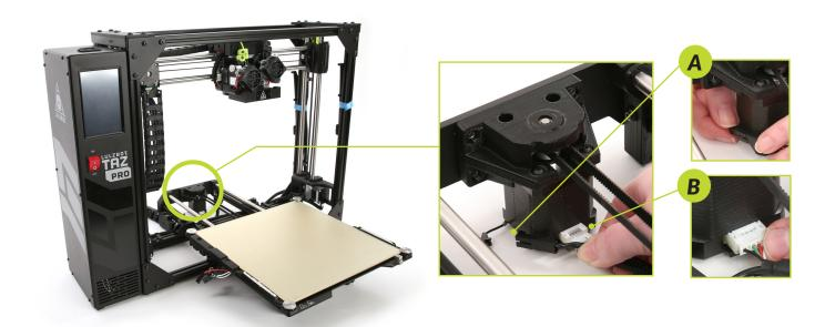
**3.7** A Connect the three sets of wire connectors underneath the bed as shown below, starting with the small two pin connection, **B** then the small three pin connection, **C** then the large heater connection.
