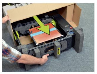
**2B** Carefully remove the protective foam piece that is supporting the Y-axis assembly.
