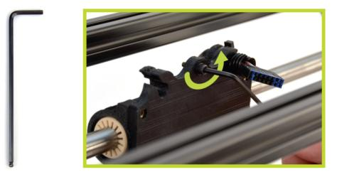
The tool head carriage is parked to the right side of the X-axis for shipping. You may want to slide it toward the center of the X-axis to make it easier to access for this step.
