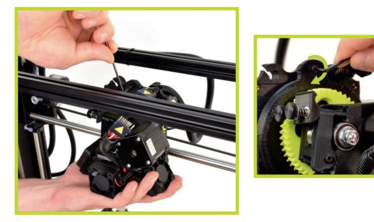
**7C** Reinsert and tighten the tool head mounting screw clockwise with the 2.5mm hex key to secure the tool head. Support the tool head with your hand to prevent it from falling onto the print surface.
