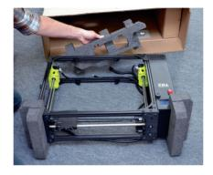
**2E** Stand the printer frame upright and remove the final two pieces of protective foam.
