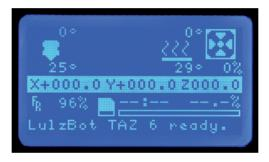
If your Graphical LCD controller shows any error messages or does not seem to power on properly, unplug the printer and then check all connections made in previous steps. Visit LulzBot.com/Support for more assistance.
