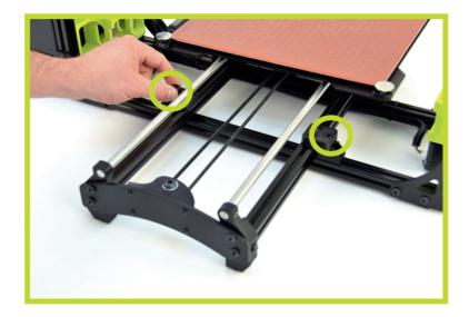
**4D** Gently slide the print surface to the front and install the two (2) rear thumbscrews. Hand tighten until snug. Do not use a tool to tighten the thumbscrews.
