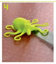
The blade is sharp, so be careful when using the blue handled knife. When in use, the knife blade should be nearly parallel with the print bed. Carefully pry away from the bed, with the sharp edge between the object and print bed.
