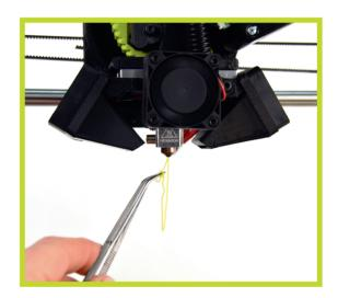
**9C** Wait ten seconds for the filament to cool, then remove the extruded filament with the included tweezers.
