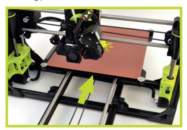
Your printer is now actively cooling. Do not attempt to remove your 3D printed object before the print bed moves forward. Attempting to do so could either burn your skin on the hot end or print bed, or damage your 3D printed object.
