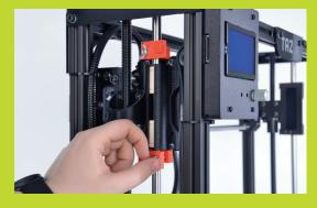
Remove red protective packing clips from Z and Y axis smooth rods.
