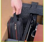
While keeping the printer in the box, pick up by the black aluminum frame and rotate the printer and foam 90 degrees - setting it upwright within the box. Make sure name plate at top is UP. Remove top foam.
