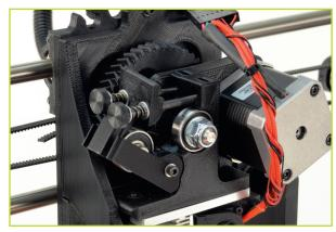
C Once the filament extrudes a small amount out of the nozzle, raise the idler and slide the two idler bolts and plate back into place. Tighten the two idler bolts. Tighten the two screws until the top of the thumbscrews are about 10–11mm away from the plastic clip.
