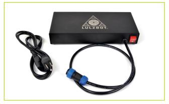
Locate the blue 24VDC output cable plug from the power supply. Connect the blue power supply plug into the keyed power supply connector on the TAZ electronics enclosure. Once the plug is pushed in completely, turn the locking sleeve clockwise until it is tight against the electronics enclosure. Hand tighten only!
