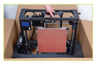
**B** Rotate printing bed assembly, tilting the bottom toward front of box. Lower entire bed into box so it is parallel with printer frame, then lift out and set aside.
