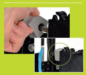
Locate and remove the gray foam block used to hold the X axis carriage in place during shipping.
