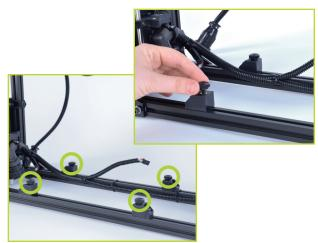
Locate the four Y axis mount brackets on the TAZ Y axis.
