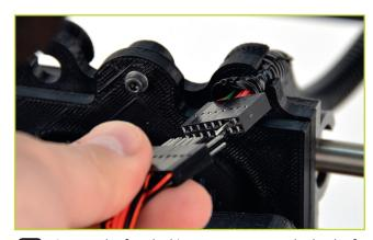
Locate the four locking connectors on the back of the electronics case enclosure. Each connector matches a keyed plug, which may require rotating the plug until the keys line up and the plug can be pushed in. Once the plug is pushed in, turn the locking sleeve clockwise until it is tight against the electronics enclosure.
