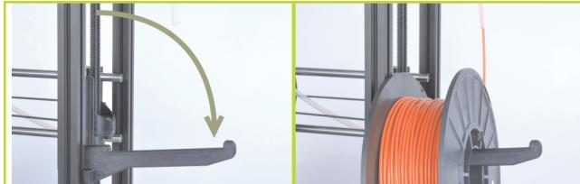
**A** Place the filament on the filament arm (front right hand side of the printer) with the filament feeding counter clockwise. Feed the filament through the filament guide, it should wind through the tube and end at the tool head.
