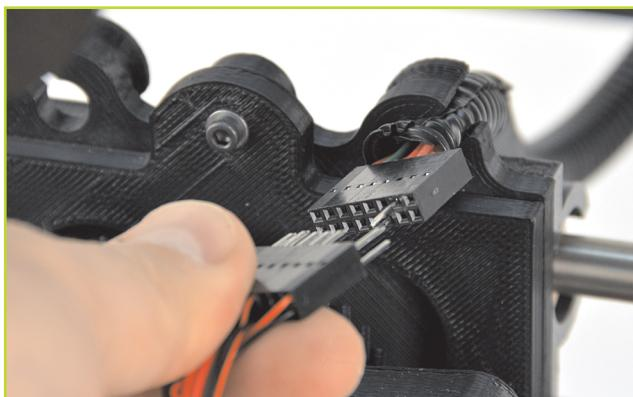
**8** Locate the four locking connectors on the back of the electronics case enclosure. Each connector matches a keyed plug, which may require rotating the plug until the keys line up and the plug can be pushed in. Once the plug is pushed in, turn the locking sleeve clockwise until it is tight against the electronics enclosure.
