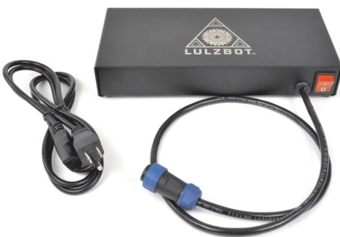
**10** Locate the blue 24VDC output cable plug from the power supply. Connect the blue power supply plug into the keyed power supply connector on the printer electronics enclosure. Once the plug is pushed in completely, turn the locking sleeve clockwise until it is tight against the electronics enclosure. Hand tighten only!
