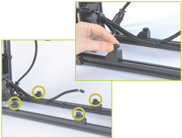
**3** Locate the four Y axis mount brackets on the Y axis.
