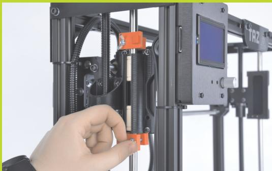
Remove the red protective packing clips from the Z and Y axis smooth rods.
