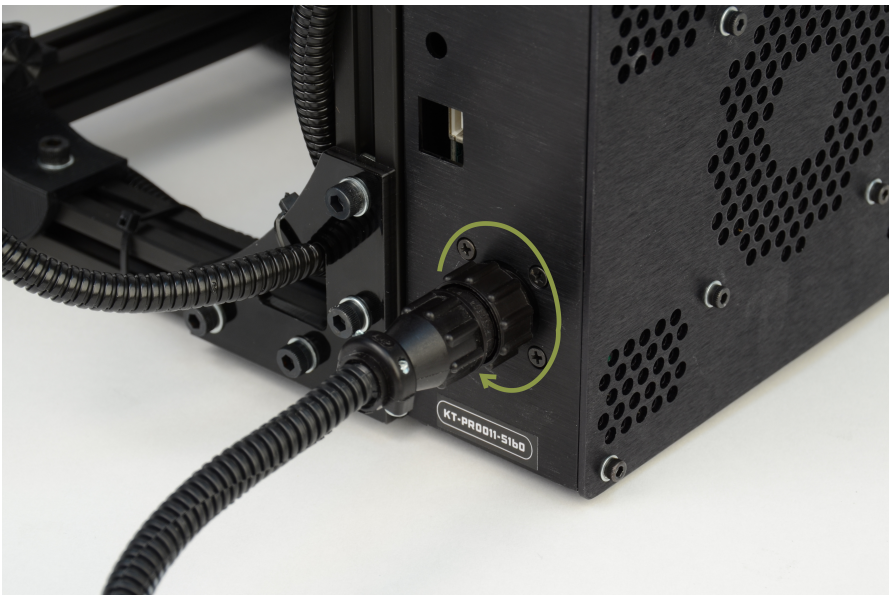
Figure 1.17: The power supply plug correctly plugged in
