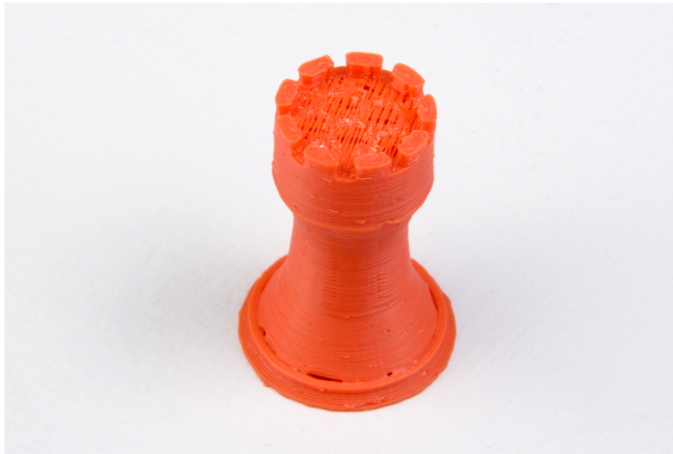
Figure 5.15: An example of insufficient top layers.
