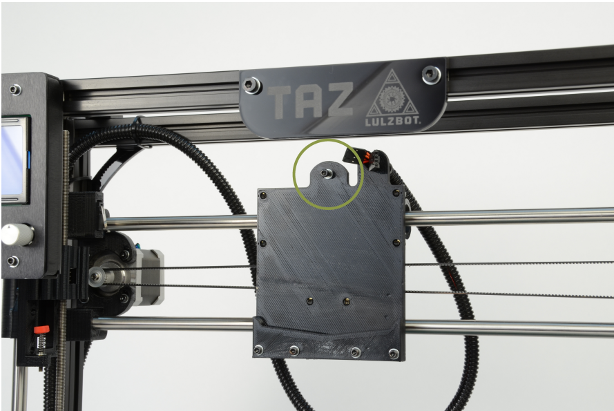
Figure 1.11: Remove the tool head screw
