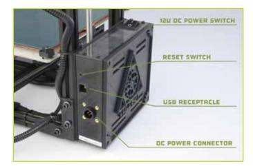
**12** Connect the DC locking plug into the DC connector on the TAZ electronics enclosure.
