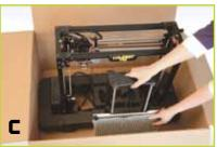
**5** While pushing down on bottom foam, carefully remove printer frame from box. Set it on a sturdy, flat surface for assembly.
