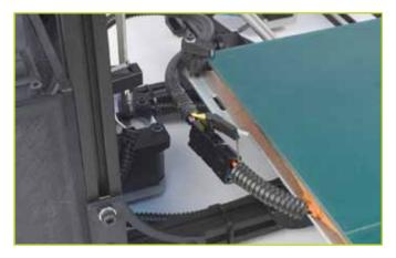
**T** Locate the two small black zip ties that are included in the documents bag. Wrap the two zip ties through the slot, located on the left rear of the aluminum bed plate, and around the print bed wires. Tighten the zip ties so the wire cannot move freely. Cut off the excess end of the zip ties with the needle-nose pliers included in the tool bag.
