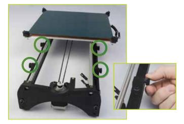
Locate the four Y axis mount brackets on the TAZ frame.
