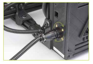
The plug is keyed which may require rotating the plug until the keys line up and the plug can be pushed in. Once you have pushed in the plug turn the locking sleeve clockwise until it is tight against the electronics enclosure.
