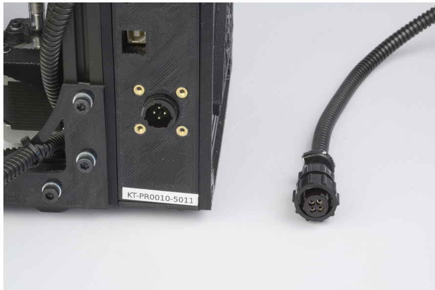
Figure 1.11: 12V DC Power supply plug and receptacle
