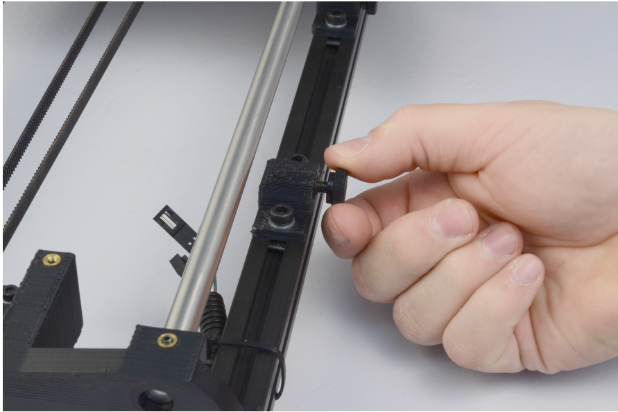
Figure 1.2: Remove the four Y axis bolts
