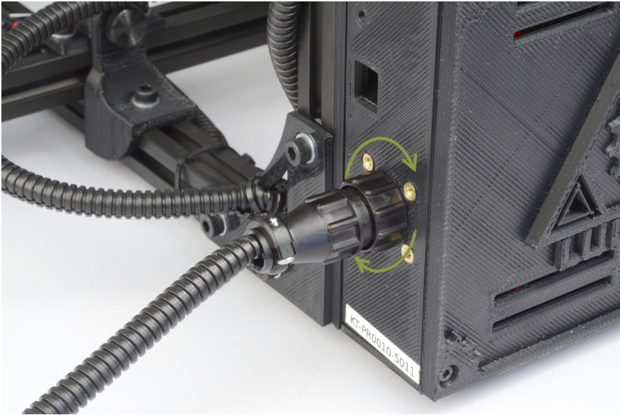
Figure 1.12: The power supply plug correctly plugged in
