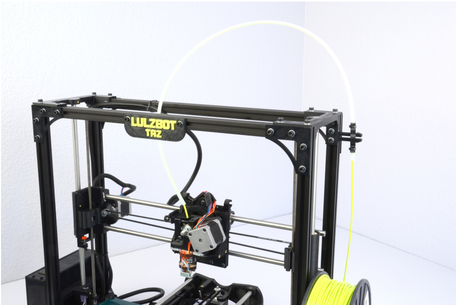
Figure 4.4: Filament run through the guide
