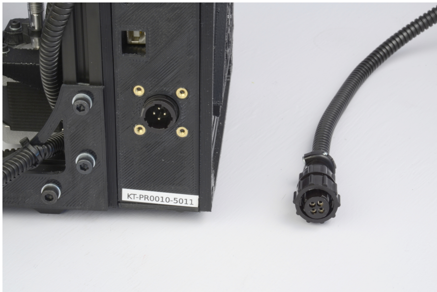
Figure 1.11: 12V DC Power supply plug and receptacle
