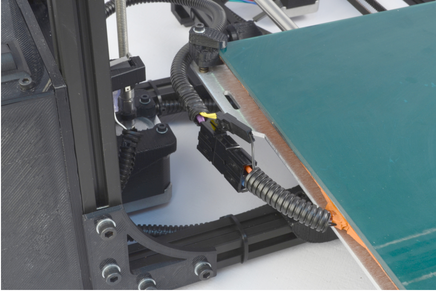
Figure 1.6: Connect the two connectors on the left of the print bed
