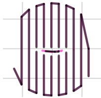
Figure 3.38: Support infill pattern: Rectilinear
