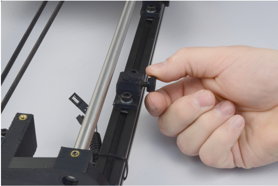
Figure 1.2: Remove the four Y axis bolts
