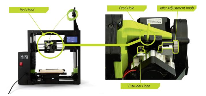
During printing, the idler holds filament against the extruder hobb which pushes filament down into the hot end. Correct idler tension is important for keeping filament flowing properly during the printing process. The idler tension can be seen by looking at the tool head from above. Rotating the idler adjustment knob clockwise will loosen the idler, while rotating counterclockwise will tighten the idler.
