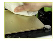
**PEI with Glue Stick:** For some filaments a polyvinyl alcohol (PVA) glue stick, such as an Elmer's® brand glue stick is necessary for bed adhesion and/or release. Apply glue stick in light, even coats. Remove accumulated glue with a damp paper towel occasionally to maintain a flat, smooth base for your 3D prints.
