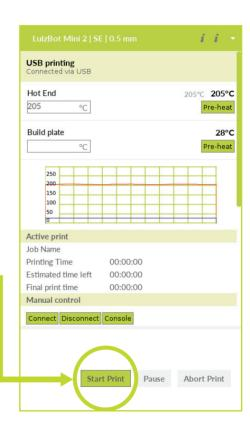
**10C** The tool head will then move to the back of the bed to clean off the nozzle. After cleaning, your LulzBot Mini will conduct an automated self-leveling sequence by touching each bed-leveling sensor, heating up to final temperature, and starting to print. This process can take approximately two to four minutes.
