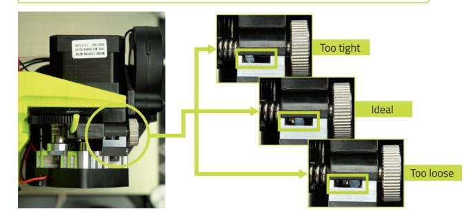
Solutions the idler as needed by turning the silver idler adjustment knob clockwise. Squeeze in on the idler and insert filament into the feed hole and all the way through the idler until it is held in place by the extruder hobb. Once the filament is in place, retighten the idler to the tension shown below with about 2 millimeters on either side of the nut as seen through the window.
