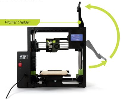
**8B** We strongly recommend using the included PLA filament sample for your first rocktopus print. Mount the PLA filament sample on the filament holder so the filament can feed down into the tool head.
