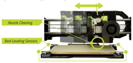
If probing fails to detect one of the bed corners, the printer will attempt self-cleaning again, then repeat probing. If this fails more than three times, or if the bed corner is visibly pushed down during probing, the printer requires manual nozzle cleaning. Refer to the Maintenance section at the end of this guide for details on nozzle cleaning.
