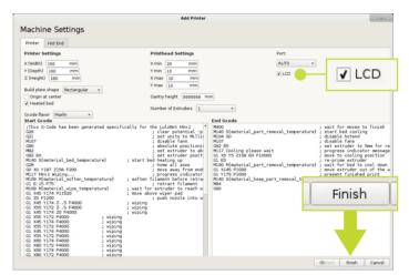
**3B** Confirm that the LCD box is checked, then click **Finish** to complete the printer setup. Cura LulzBot Edition is now ready for use with your LulzBot Mini 2.
