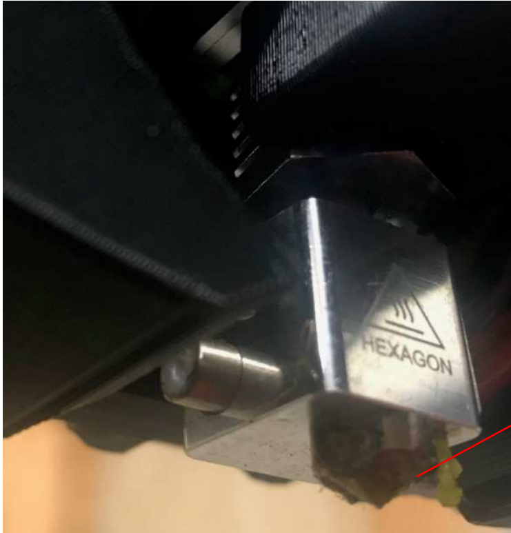
Photo 3- View of the extruder heater
