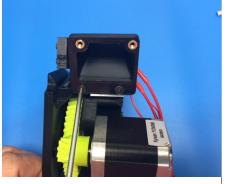
60) Connect the Hexagon Hot End ground wire (220mm long) to the hot end. Route the ground wire behind the hot end, Plug ground wire into the 16pin connector that is attached to the motor.
