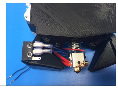
130) Attach Heat Sink Fan Duct to assembly
