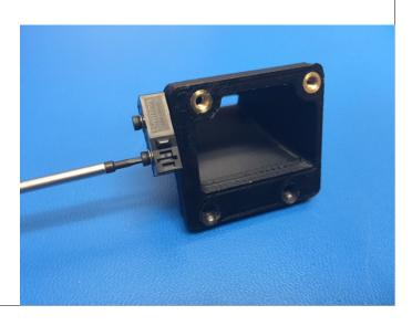
30) Prepare the Hexagon heat sink fan and attach to the Hexagon Hot End Heat Sink fan duct (PP-GP0232) with inserts already installed. Note orientation of fan. Use: 4x- M3x 12 SHCS tighten to 8 in-lbs (~.9N-m)
