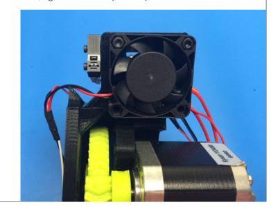
120) Connect Switch to the 16 pin connector, connect to the switch terminals shown; route wires as shown
