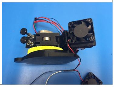
110) Route the long fan wire along the back of the mount, secure in place with a Ty wrap as shown, proper routing is critical
