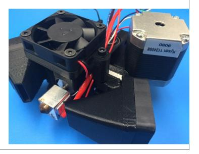
140) Attach Heat Sink fan to 16 position connector Wrap 3/4" panduit (110mm length) around wires starting at the bottom of the connector and completing as far down the wire bundle as possible Secure the panduit to the wire bundle with one Ty Wrap; Position the Ty Wrap approximately where shown
