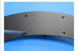
Start the first two screws in opposite corners before installing the last two screws and tightening all four
