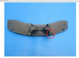
Gather- Motor side parts Align motor mount (with inserts already installed) to plate
