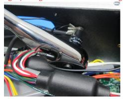
30) Install Interconnect Housing on case exterior, verify slot in interconnect Housing aligns with slot in case
