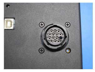
16) Position the EL-MS0144 (Sealing Cap) strap so the strap will double over itself when the cap is installed onto the 16position round connector, secure the sealing cap with 1x- 18-8 FHS Black Oxide; tighten to finger tight, the cord should not be able to rotate once
