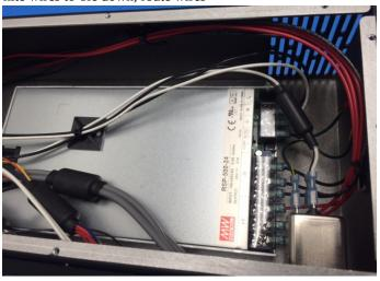
29) Install **1x-M3 star washer** to the case ground lug near the RAMBo, install 7 ground wires from the internal cable harness to the ground lug, secure with **1x-M3 Nyloc nut tightened to hand tight (if using a ratchet beware of over-tightening the nut)**
