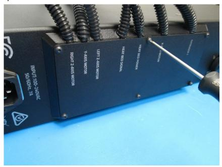
35) Inspect wiring layout to ensure all connections are made and wires are laying correctly
