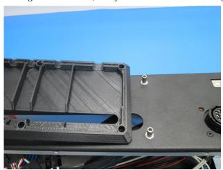
31) Route connectors from each of the internal harnesses into the Interconnect Housing, connectors sizes indicate proper position in the Interconnect Housing
