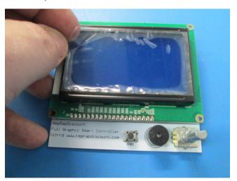
9) Install printed LCD spacers into LCD assembly screw mount hole locations (4x), Install **4x- M2.5x12 SHCS and 4x- M2.5 washer-** Align LCD with mounting standoffs- **install screws to finger tight + necessary turns to ensure the LCD is secured and cannot move**
