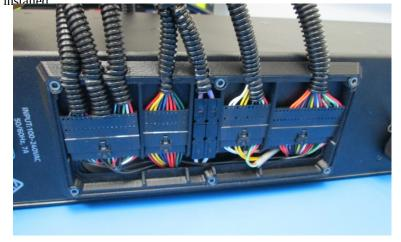
34) Install interconnect housing cover with 6x- M3x12 BHCS and 6x- M3 washer; tighten to hand tight; ensure the cover is flush to the interconnect housing and the interconnect housing is flush to the case. DO NOT TIGHTEN screws past hand tight to force either the cover or the interconnect housing into place.
