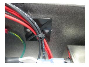
24) Route Red and Black Power Supply wires to second tie down, ensure sufficient service loop and bend radius is maintained (see picture), secure wire with Ty Wrap with the securing latch positioned toward the case opening
