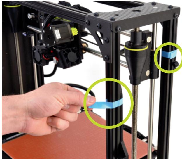
**9B** Rotate filament reel holder and guide tube bracket clockwise into position.
