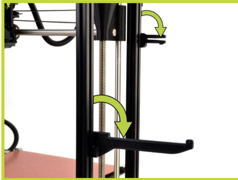
**9C** Slide filament guide tube onto the bracket.
