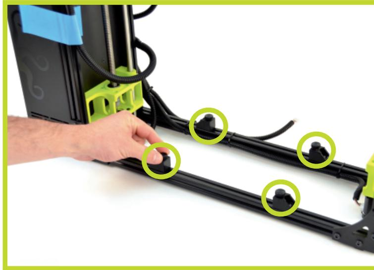
**4B** Set the Y-axis assembly onto the base of the printer frame, carefully lining up the four (4) mounting brackets. The print bed wiring should be on the left side as shown.
