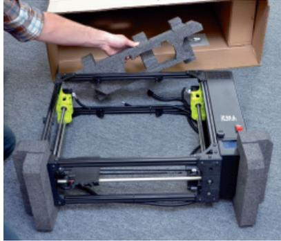
**2E** Stand the printer frame upright and remove the final two pieces of protective foam.
