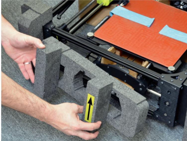
**2C** Lift the front of the Y-axis assembly up, then pull it out of the 3D printer frame. You may need to push the Y-axis assembly back before lifting so that it clears the frame.
