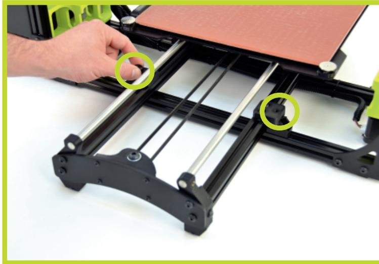
**40** Gently slide the print surface to the front and install the two (2) rear thumbscrews. Hand tighten until snug. Do not use a tool to tighten the thumbscrews.
