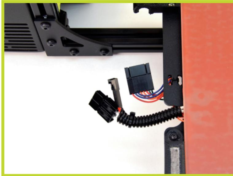
**50** Connect the three sets of corresponding wire connectors, as shown below.
