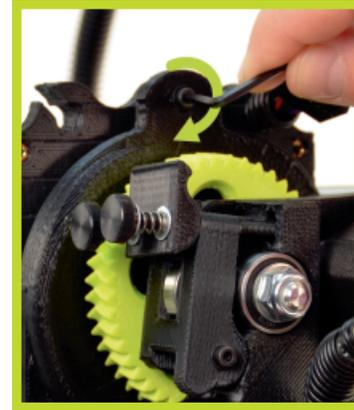
**7C** Reinsert and tighten the tool head mounting screw clockwise with the 2.5mm hex key to secure the tool head. Support the tool head with your hand to prevent it from falling onto the print surface.
