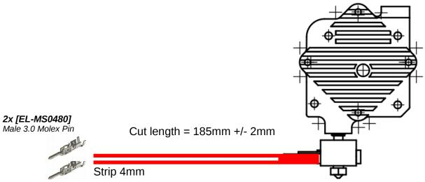
Both conductor and insulation crimp are to be on the conductor only. Do not crimp the insulation.
