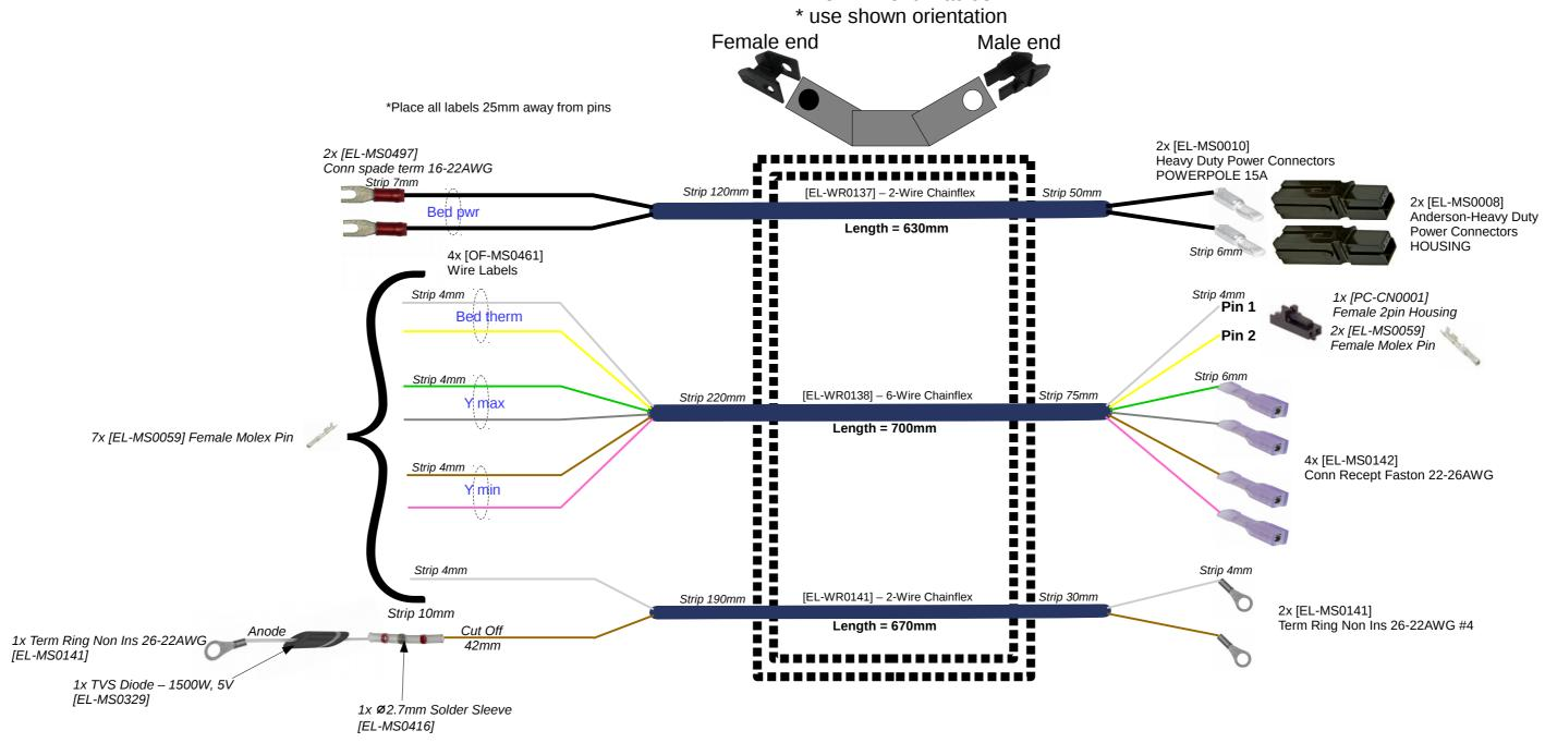
Cut Tolerance:  $\pm 3.175 \frac{\text{mm}}{0.3048 \text{m}} \pm 1.041 \frac{1}{66} \%$
