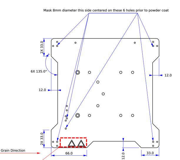
Part is to be laser etched in the indicated area.
