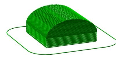
Figure 3.53: Example with variable layer height.
