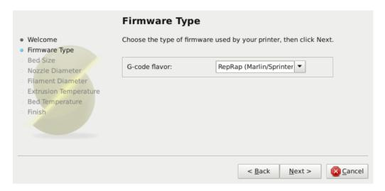
Figure 3.2: Configuration Wizard: Firmware Type
