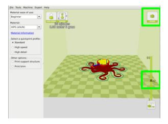
Figure 2.10: Viewing Specific Layers
