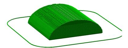
Figure 3.55: Example with skipped layers.
