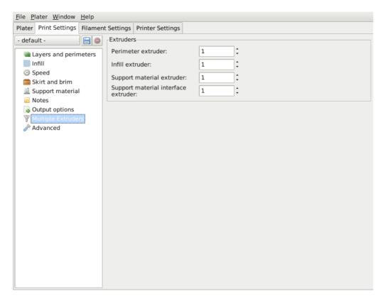
Figure 3.46: Multiple extruder options - Print Settings Tab.
