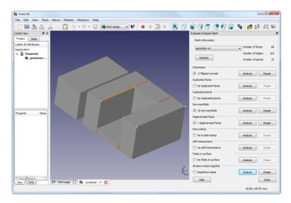
Figure 3.58: FreeCAD part repair.
