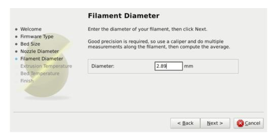
Figure 3.5: Configuration Wizard: Filament Diamter
