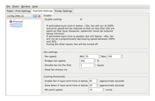
Figure 3.36: Cooling advanced settings.
