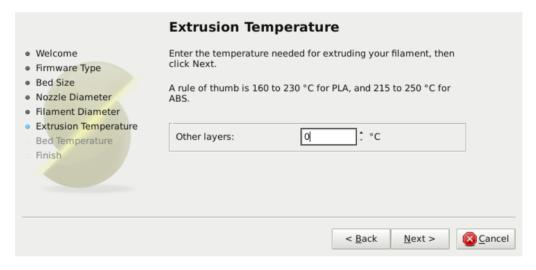
Figure 3.6: Configuration Wizard: Extrusion Temperature
