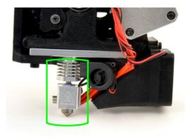
Figure 3.60: The clearance cylinder around an extruder.
