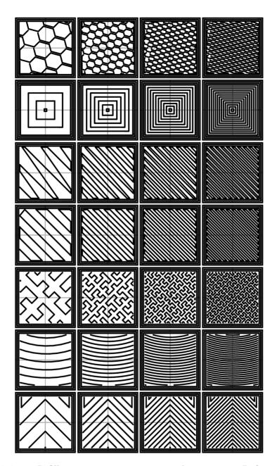
Figure 3.31: Infill patterns at varying densities. Left to Right: 20%,40%,60%,80%. Top to Bottom: Honeycomb, Concentric, Line, Rectilinear, Hilbert Curve, Archimedean Chords, Octagram Spiral
