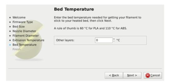
Figure 3.7: Configuration Wizard: Bed Temperature
