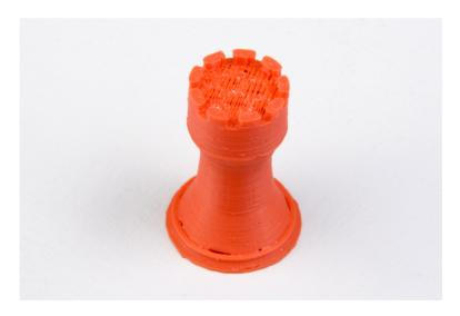
Figure 3.15: An example of insufficient top layers.
