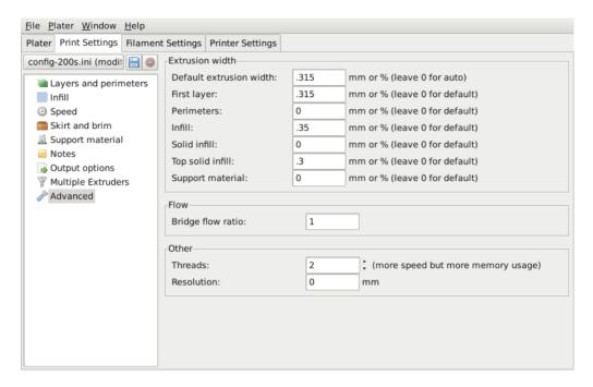
Figure 3.48: Extrusion widths options.
