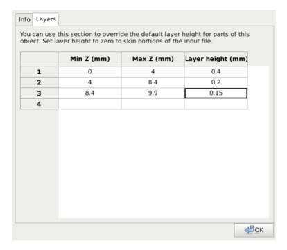
Figure 3.52: Variable layer height options - Layers.
