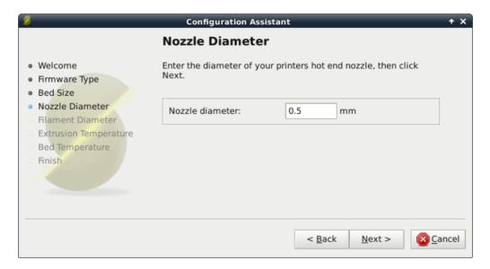
Figure 3.4: Configuration Wizard: Nozzle Diameter
