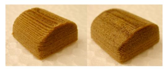
Figure 3.54: Example print with variable layer height.
