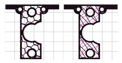
Figure 3.30: Infill pattern comparison in a complex object. Left to Right: honeycomb, line
